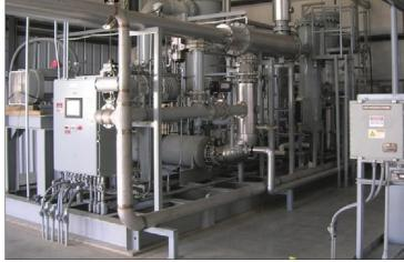
The City of Billings, Montana landfill wanted to monetize their landfill gas through upgrading to pipeline standards. The feed gas from the landfill necessitated removal of both N2 and CO2. The solution chosen is a Guild Associates' Molecular Gate™ Pressure Swing Adsorption (PSA) system using two PSAs in series, the first removes CO2, followed by N2 removal.
