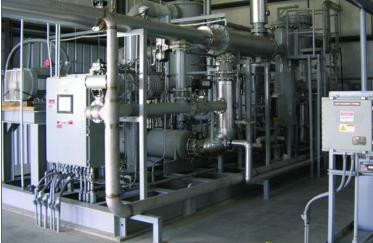
Guild Associates' Molecular Gate<sup>TM</sup> Pressure Swing Adsorption (PSA) systems will remove the target gas (CO<sub>2</sub> or N<sub>2</sub>) plus water, volatile organic chemicals (VOC), hydrogen sulfide and siloxanes in a single-step process. This is accomplished without the use of disposable media, as the Molecular Gate adsorbent is not replaced during the lifetime of the equipment.
